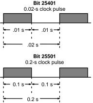
Because the 0.1-second and 0.02-second clock pulse bits have ON times of 50 and 10 ms, respectively, the CPU may not be able to accurately read the pulses if program execution time is too long.
